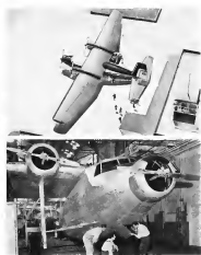
Trimotor Cargo Plane: Northrop Aircraft's Pioneer, conventional passenger and cargo transport, shown in artist's sketch and in mockup designed specifically for use as rugged carrier, it has a high payload, fixed landing gear and exceptionally short take-off and landing distances. Prototype is nearing completion.
